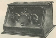
The panel view of the receiver that employs the Roberts circuit. Photos courtesy of Hammarlund-Roberts.
