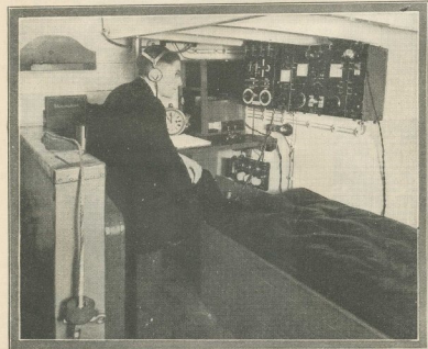
Interior of wireless cabin, showing Radio Operator Gilbert Moss, seated before his instruments. Behind him, on the deck, is the loop antenna, unshipped. In the corner of the bench is the \frac{1}{4} K.W. quenched spark transmitter, and on the bulkhead in front of Mr. Moss is the 6-tube radio compass receiver and the 2-tube all-wave receiver, both fitted for alternative crystal operation. Photos © Marconi Wireless Telegraph Co., Ltd.
