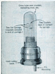
The crystal detector shown here is described above. The photograph is nearly full-size.
