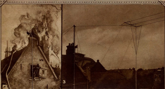
No. 1. The fireman on the roof carries a reel of wire on his back to which is connected a microphone, into which he reports the progress made in the fire-fighting. This is put on the air by means of the portable transmitter, shown at No. 2, which is at the scene of the fire. The message is received at the central fire station, the antenna of which is shown at No. 3. The system is so arranged that three fires can be reported upon simultaneously. The receiver and transmitting equipment is shown in No. 4. Photos Courtesy of "Fire and Water Engineering," (New York.)
