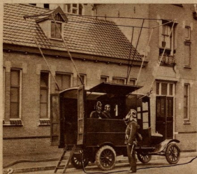
No. 1. The fireman on the roof carries a reel of wire on his back to which is connected a microphone, into which he reports the progress made in the fire-fighting. This is put on the air by means of the portable transmitter, shown at No. 2, which is at the scene of the fire. The message is received at the central fire station, the antenna of which is shown at No. 3. The system is so arranged that three fires can be reported upon simultaneously. The receiver and transmitting equipment is shown in No. 4. Photos Courtesy of "Fire and Water Engineering," (New York.)
