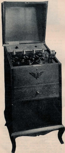
Fig. 5. This four-tube receiver, installed in a phonograph cabinet and using the Flewelling circuit attracted much attention at the exhibit.
