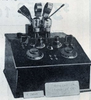
Fig. 3. A two-tube reflex that attracted great attention.
