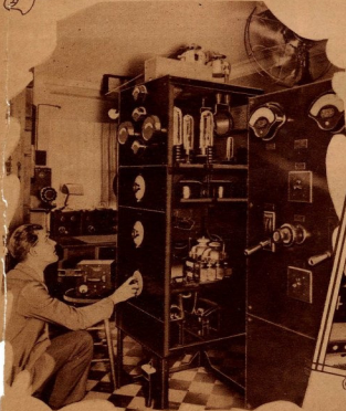
THE TRANSMITTER AND CONTROL PANELS. In the transmitter can be seen the large tubes and tuning apparatus and on the right is the panel on which is mounted the apparatus which controls the motor generator set.
