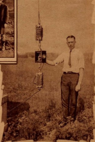
THE ANTENNA METER. This meter is in the lead that goes from the transmitter to the antenna and is quite a distance from the building where the transmitter is located, so that the readings are taken with the aid of a telescope.
